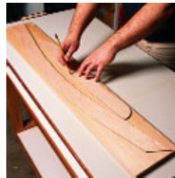
Trace your pieces onto cedar from your template. Be as space-efficient as possible. Cut out each of the pieces with a bandsaw. A scrollsaw or jigsaw also does the job.
