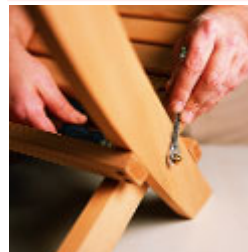
Install the brass bolts, washers and cap nuts to join the seat supports to the backrest.
